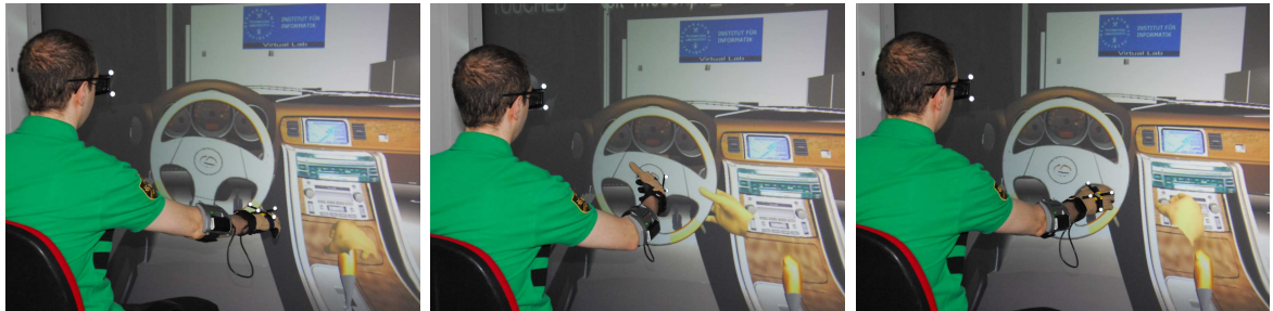
Figure 7.16: Recording session for action capture: the human demonstrator wears a dataglove and tracking markers and performs a set of manipulations in a virtual cockpit of a car. First he grasps the gearshift, then the steering wheel and, finally, the radio button.
