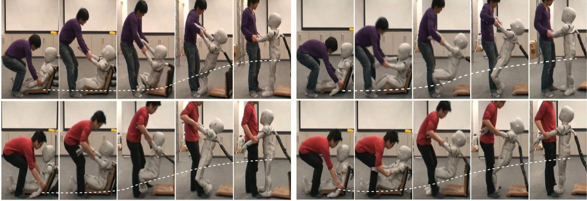
Figure 6.23: Sequential photographs of the first (top) and last (bottom) interactions of the test subjects with the robot. The white curve depicts the change in position of the robot’s hips. The center photograph of each sequence shows how the robot learns to maintain firm contact between its feet and the ground for both subjects.
