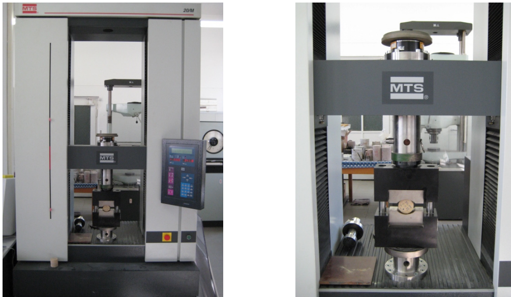
Figure 3-7: Loading jaws of rock mechanics test system MTS 20/M (3) .
