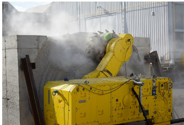
Fig. 1: Rock cutting test bench in Czech Republic
