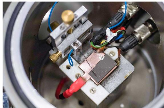
(d) Sample stage with adjustable needle contact for small contact pads. See also Fig. 4.3(b).
