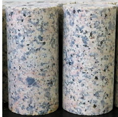
Figure 3-2 Cylindrical sample of Eibenstock granite at room temperature
