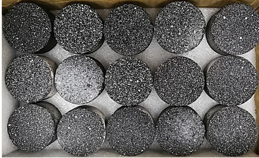
Figure 4-2 Some Brazilian discs with white spots sprayed on the thin black opaque layer
