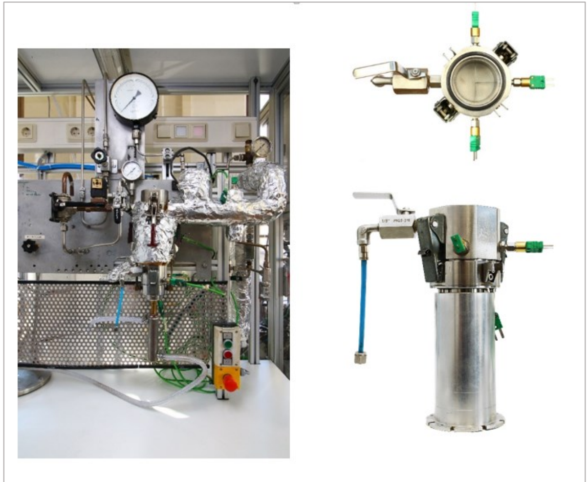
Figure 47. Steam pressure filtration apparatus [12, 13].
