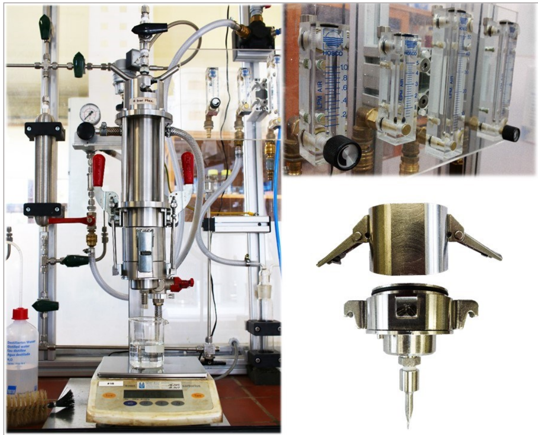
Figure 44. Images for the Nutsche apparatus (according to VDI 2762-2) [18].
