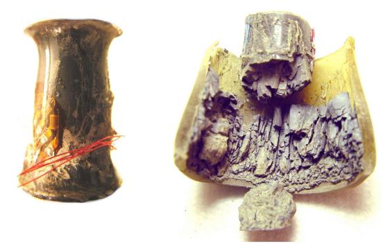
Figure 18 Failed SiC sample after triaxial test: left, confining pressure P = 350 MPa, axial stress  $\sigma_a = 6514$  MPa; right, confining pressure P = 200 MPa, axial stress  $\sigma_a = 6326$  MPa. (Lee et al. 2005)
