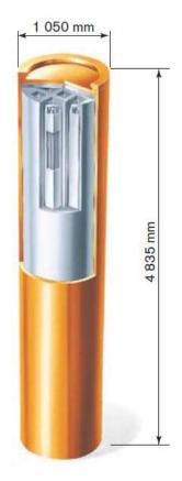
Figure 10 Swedish copper canister with cast iron insert (Raiko et al., 2010)
