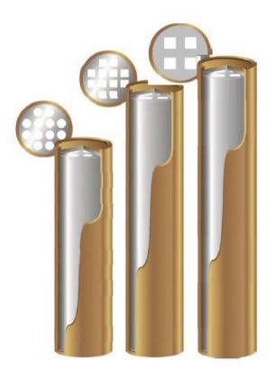
Figure 11 Finnish copper canister: heights are 3.6 m, 4.8 m, and 5.25 m (from left to right) (Nolvi, 2009)
