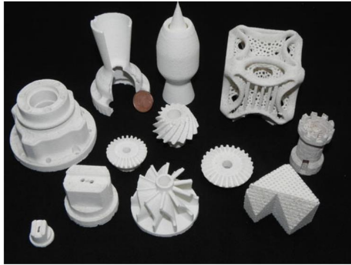
Figure 6: Pure PBF-LB processed alumina parts manufactured by Juste et al. [50]
