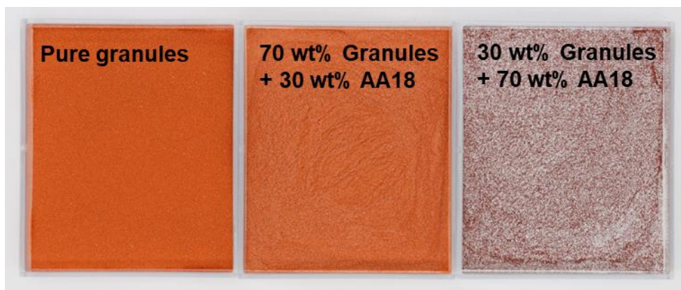
Figure 58: Powders to evaluate the influence of coarse alumina variation on the part formation by PBF-LB.
